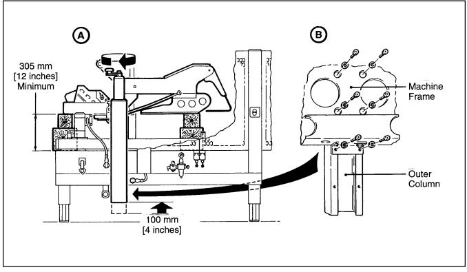
Figure 6-4 – Column Re-Positioning
